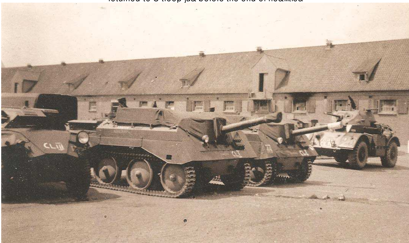
Image courtesy of the Trooper Alfred William Bolden who served between 1942-1947. Description: Having had the turrets removed to be fitted onto the Daimler heavy armoured car, these Tetrach light tanks were reconfigured to accommodate a heavy gun and were designated Electra's. This photo at the end of the war shows them lined up for disposal, The Humber scout car is Class III (poor condition and probably destined for scrapping), and the electras both Class I (good condition).
