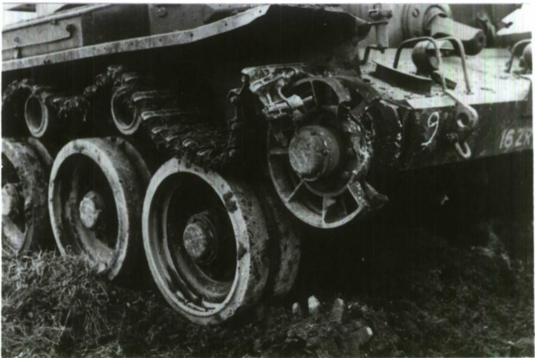
FIG. 22 DIRECT HIT ON TRACK OVER IDLER
