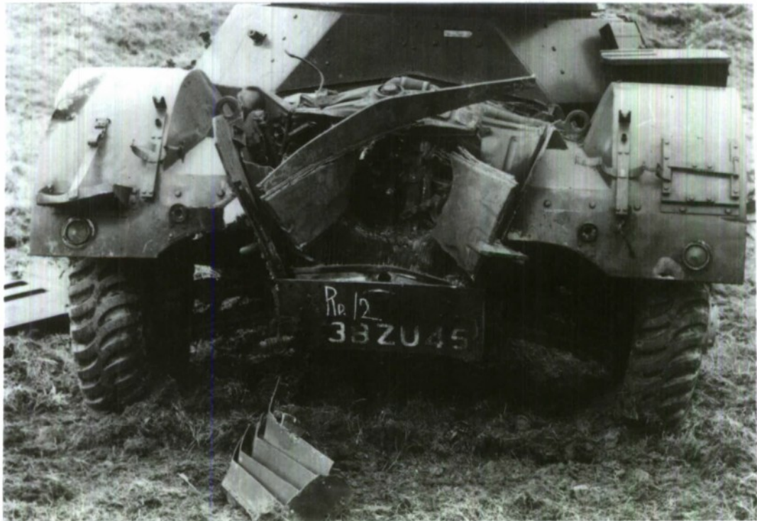
FIG. 13 DIRECT HIT ON REAR OF ENGINE COMPARTMENT
