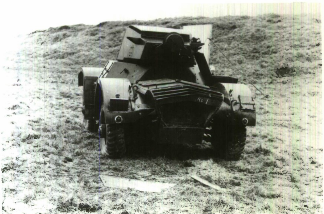
FIG. I NEAR MISS CLOSE TO THE ENGINE COMPARTMENT
