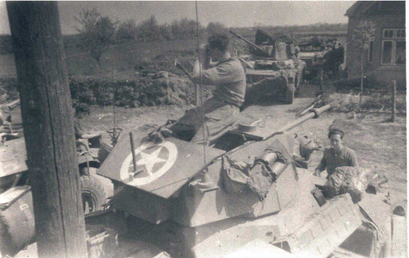
pictures courtesy Martyn Tasker (unknown source) A Daimler Armoured Car of 11 Hussars, fitted with a little john adaptor. Circa 1944
