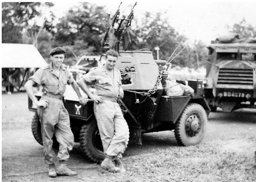
Image courtesy of Angus Mac Vicar Photographer: Alfred Cook REME Description: Daimler Dingo all tooled up and ready for patrol - GM C15TA Armoured Truck behind At Nee-Soon, Malaya Date: July 1955
